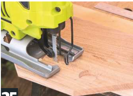
25 Remove remaining waste between holes with jigsaw. Use this for sawing tapered edges of handle
